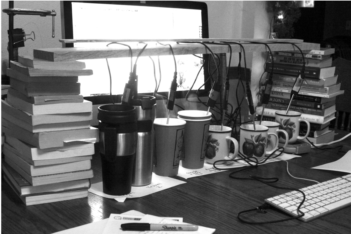
Figure 2. The eight cups with temperature probes
